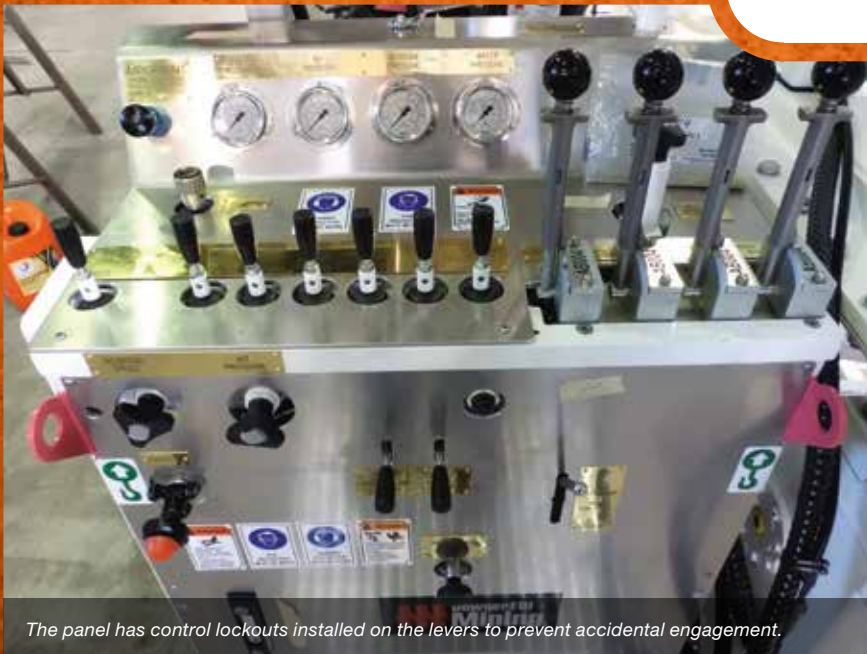
The Downer Mining-specified Alton Fly Rig complete with the new controls.
