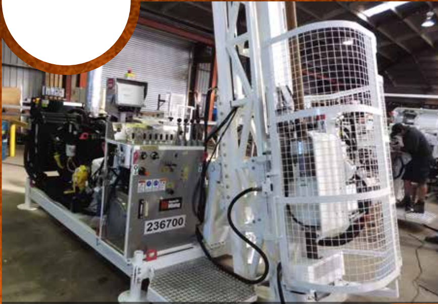
The Downer Mining-specified Alton Fly Rig complete with the new controls.
