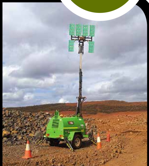
One of our lighting towers using LED lights at the Karara Iron Ore Project.
